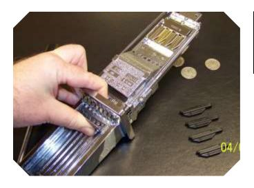
3) After pushing in the chute and your coins drop out, you will be able to access the inserts, and a section that may contain spare inserts. While holding the handle in as shown...
