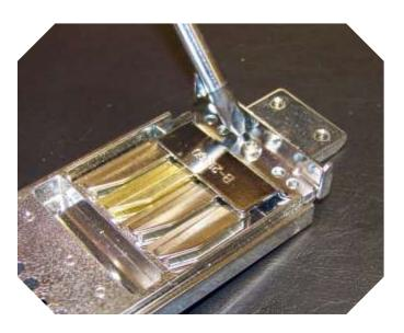
5) now you can remove the single Phillips screw holding the spring bracket to access the spare inserts (if any). This will also be a very good place to store any inserts you remove during this process so you will easily be able to find them for future adjustments, and aren't having to dig in your workbench, toolbox, desk drawer, etc..
