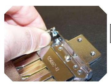
4) ...unhook the two large return springs from the small hooks on the spring bracket.
