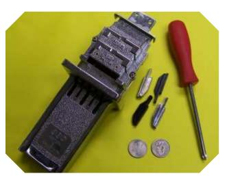
Remove the Push Chute from the coin door, and remove the push chute end, proximity plate, anything bolted to the end—for easier access. You will need the Push Chute (of course), enough coins to make it work in its current setting, the inserts for the desired setting, and a Phillips screwdriver.
